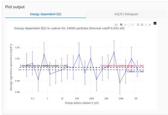
(a) Average energy decrement \xi vs. incident energy, showing the thermal transition.
